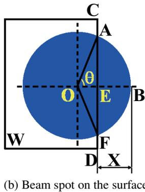
Fig. 1. Geometrical relationship of spot area across the edge.
