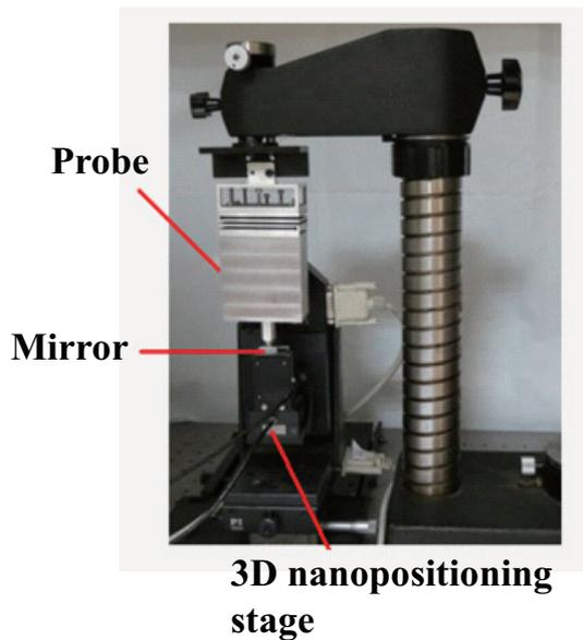
Fig. 8. Experimental setup of the measurement system.
