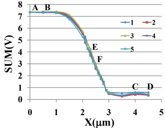
Fig. 10. Measured light intensity across the edge.
