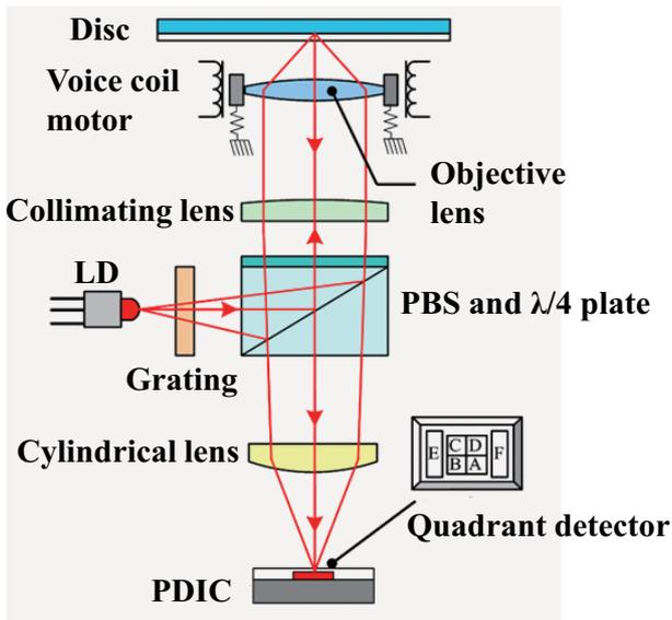
Fig. 5. Optical structure of a DVD pick-up head.
