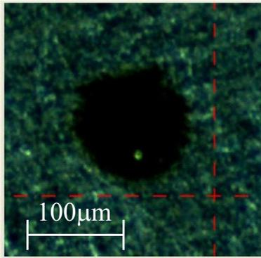
**Fig. 15.** 100  $\mu\text{m}$  pinhole with a damaged edge.
