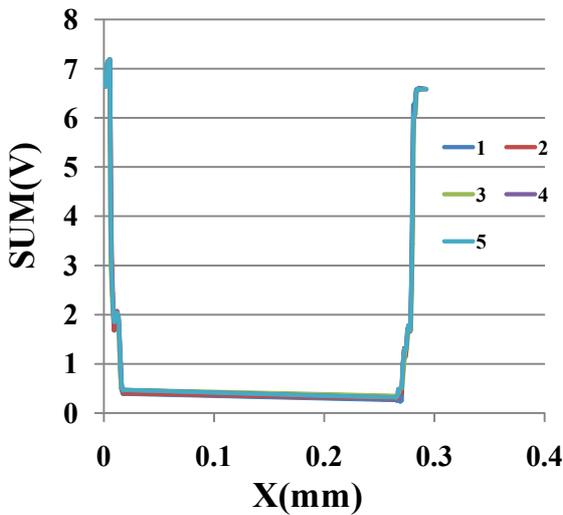
Fig. 12. Measured light intensity across the trench.
