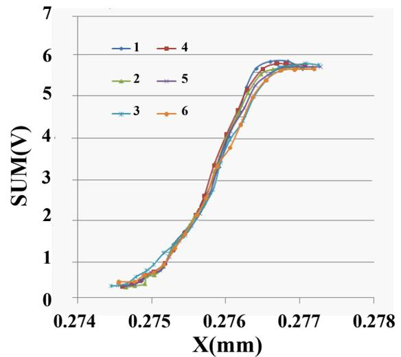
Fig. 14. Measured light intensity across the right edge.
