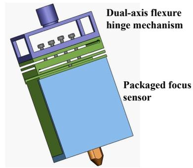
(a) CAD design of the probe
