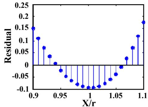
Fig. 4. Linearity error in the region of (0.9, 1.1) of X/r.
