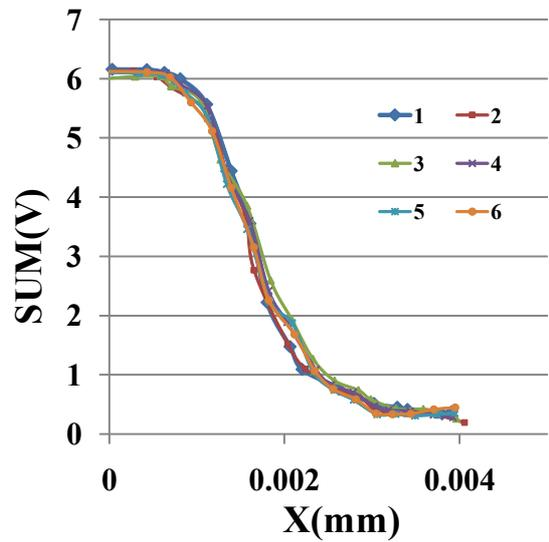
Fig. 13. Measured light intensity across the left edge.
